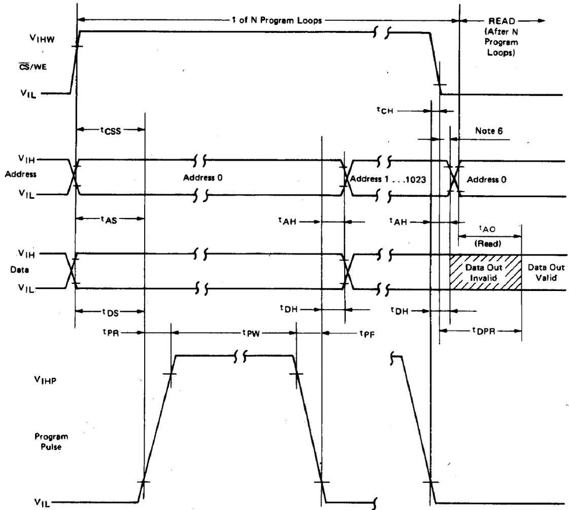
Note 6: The  $\overline{CS/WE}$  transition must occur after the Program Pulse transition and before the Address Transition.
