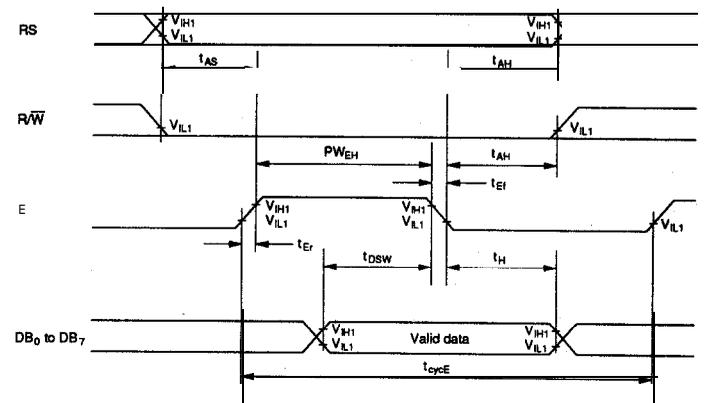
DATA WRITE FROM MPU TO MODULE
